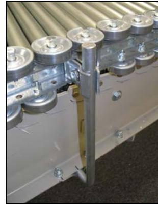
**Figure 2 – Adjustable Guard Rail**
