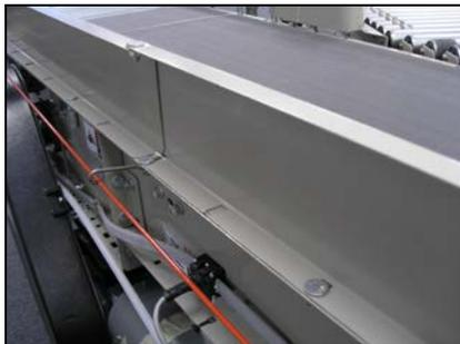
**Figure 3 – High (Channel) Fixed Guard Rail (shown without spacers)**
