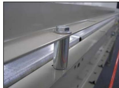
**Figure 4 – Low (Angle) Fixed Guard Rail (shown with spacers)**
