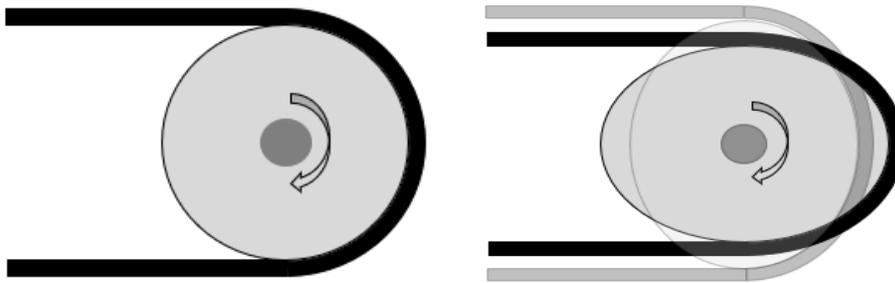
Figure 2: Drive pulley with no run-out (Left) excessive run-out (Right) [exaggerated]
