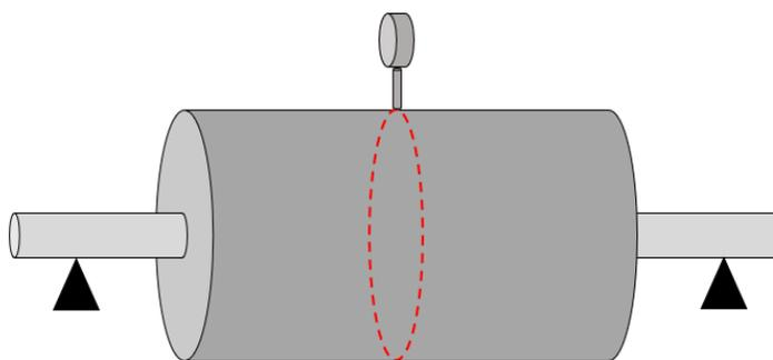
Figure 1: Circular run-out measurement on conveyor pulleys
