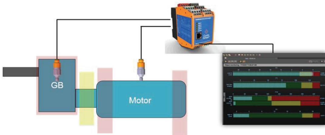
Figure 1: Monitoring System with Two Sensors and an Electronic “Brain” Sending Signals to an HMI
