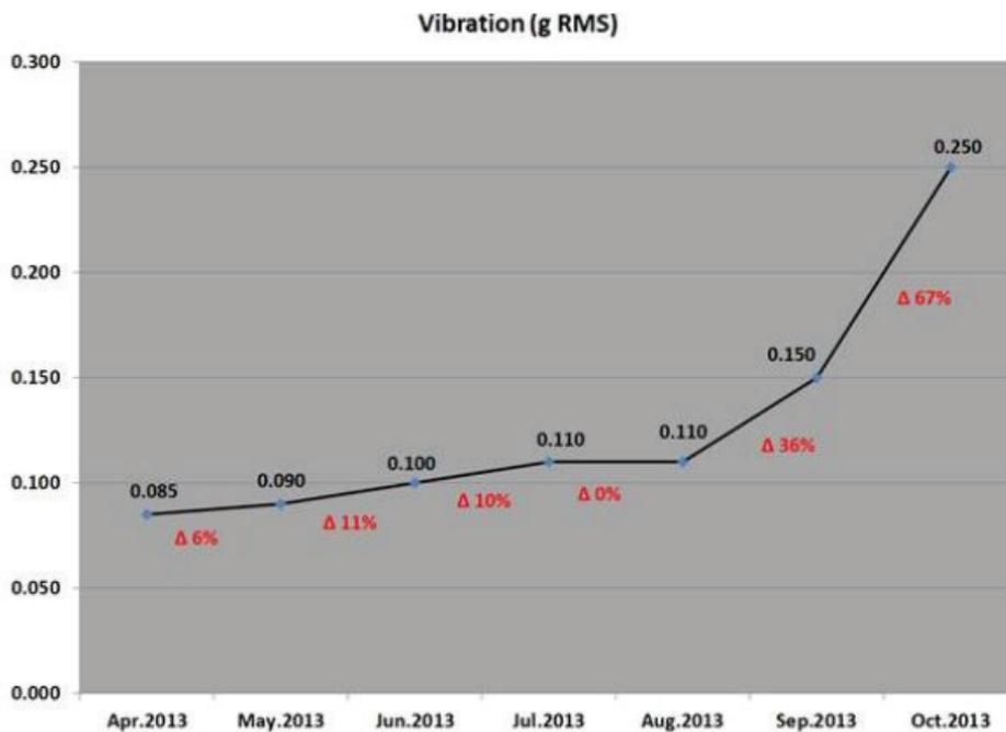
Figure 4: Example of an Upward Vibration Trend in a Gearbox
