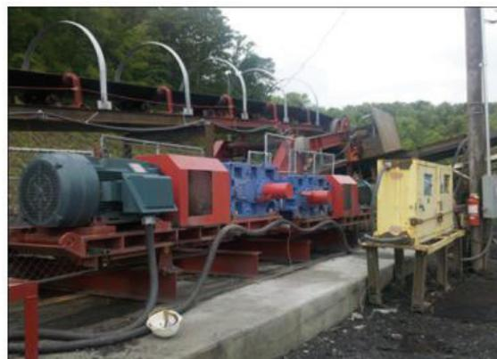
Figures 2 and 3: A typical belt conveyor with a close up of the motor and gear drive assemblies
