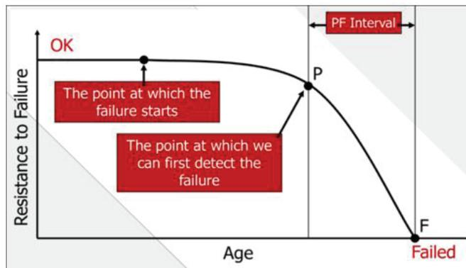
Figure 1: Typical Product Failure (P-F) Curve
