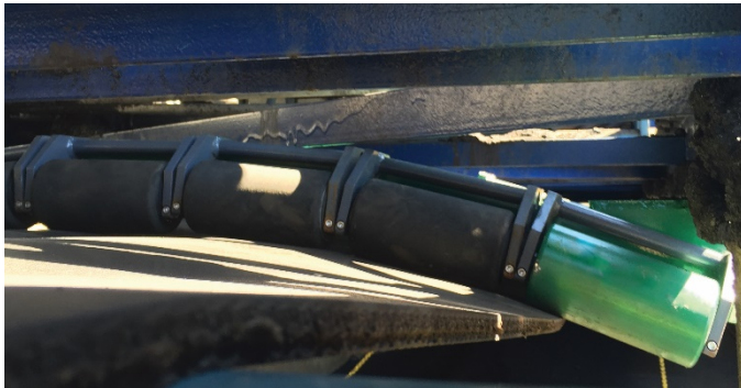
Inverted Arc Return Belt Trainer
